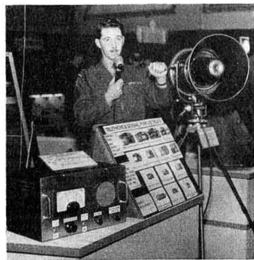
[War Office photograph In this picture, the communications receiver built by G3AMO is in the left foreground and an electro-mechanical loudspeaker to the right.
